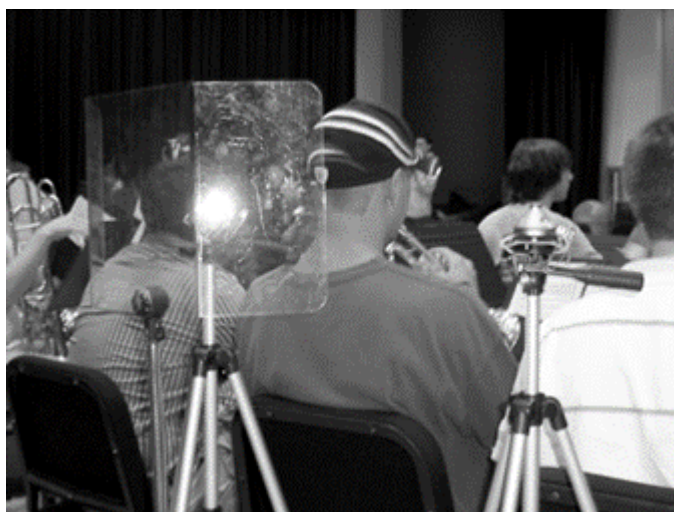
Figure 1. North Carolina Symphony shield with dose Badges, shield-protected and not shield-protected, for sound-level measurement.
