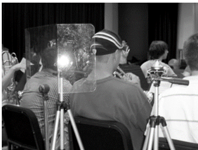
Figure 1. North Carolina Symphony shield with dose Badges, shield-protected and not shield-protected, for sound-level measurement.
