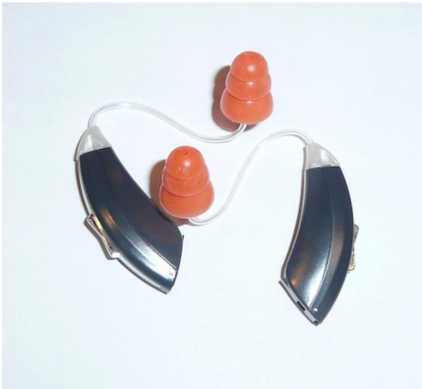
Figure 10. Clik Shooter combined earplug and amplification device. The gain option selected by the user is programmed into the device, and assists in determining the output level at which the earplug
