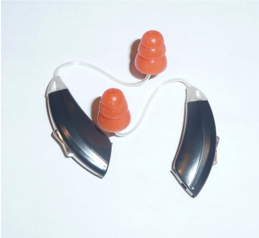
Figure 10. Clik Shooter combined earplug and amplification device. The gain option selected by the user is programmed into the device, and assists in determining the output level at which the earplug function is activated.
