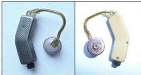
Figure 3. The Dahlberg Magic Ear II, a behind-the-ear hearing aid having an external receiver. The case was composed of two different materials. The outer shell was made of metal and the inner surface was a hard plastic. It is speculated that this was done to prevent moisture penetration and rust prevention.
