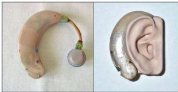
Figure 1. Zenith “Diplomat” hearing aid developed in 1956. It covered the entire area behind the auricle, from top to bottom (and a little beyond), as shown in the right image. The right image does not show the external receiver.
