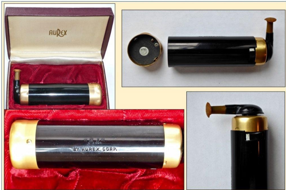
Figure 1. Aurex “P-A” (Personal Amplifier). It was advertised for use at concerts by individuals with normal hearing, but certainly would have helped those with hearing loss as well.
