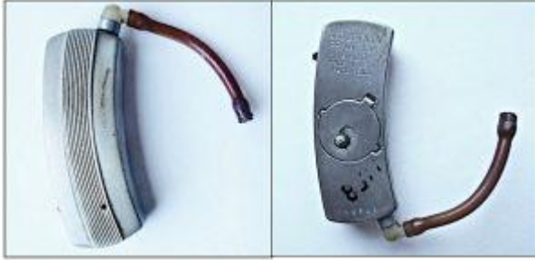
Figure 7. The Acousticon “Privat-Ear” A600 is shown front (left) and back (right). The case is made of metal, both sides. The Acousticon name and model number are shown at the top (right image). The serial number is stamped into the area near the sound tube (right image).
