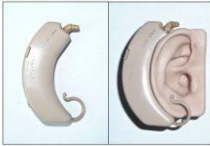
Figure 4. The Maico AG BTE hearing aid having all the components, including the receiver, housed within the case, and showing how it fit individuals. In the images shown in Figure 4, the tubing from the sound outlet nozzle (top extension) to the earmold in the ear, is missing.
