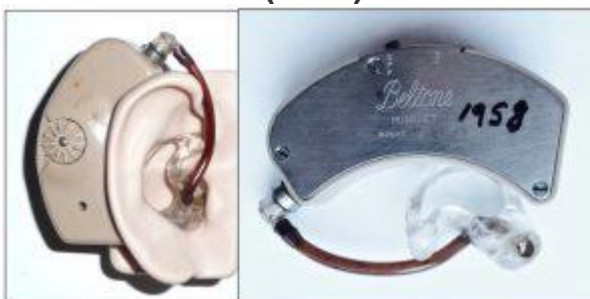
Figure 6. The Beltone “Minuet” BTE hearing aid. The unit shown is for the right ear (“Right” imprinted into the inner metal plate). It had a large volume control and a separate ON/OFF switch. The microphone opening is in on the lower, outer surface.
