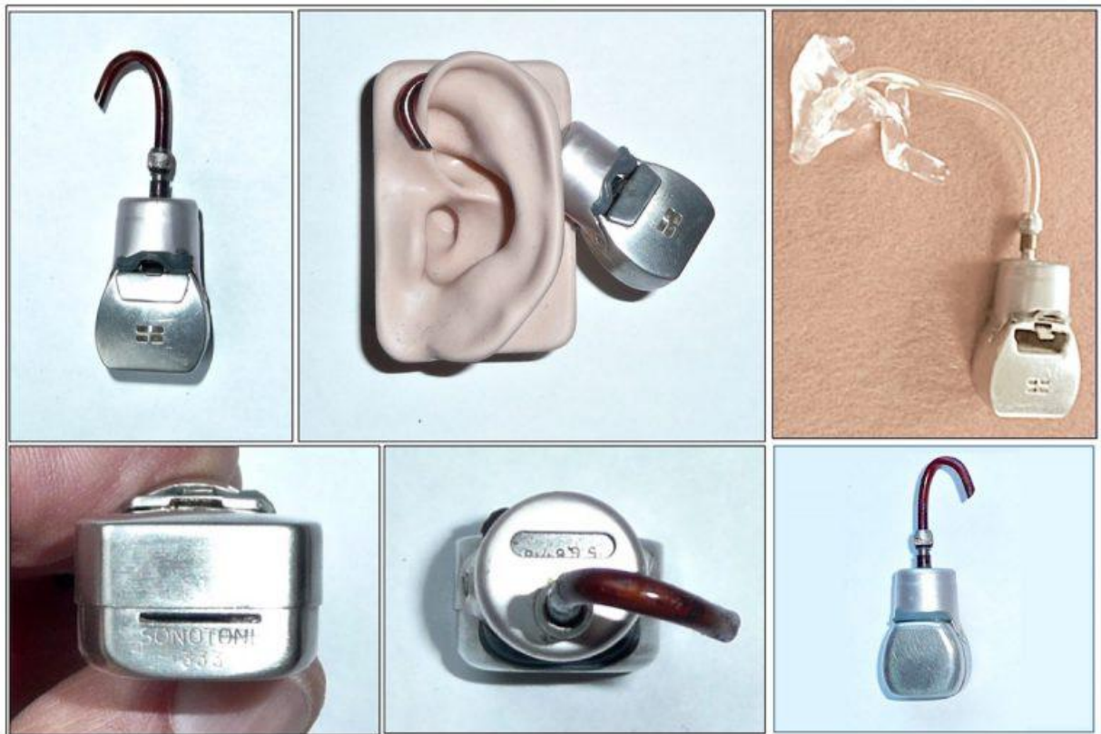
Figure 5. The Sonotone 333 BTE hearing aid. All the components were housed in a metal case. With a longer tubing than shown, the aid would hang down below and behind the lower part of the auricle, not pushed out as shown in the upper center photo. That photo is used primarily to gauge the size. The body was narrower in one dimension than the other, and when fitted with the narrow dimension against the skull, slightly limited the protrusion of the auricle caused by the aid. Again, I did not want to change any of the parts of the aid, including the tubing to the ear. The upper right image shows how it would be attached to an earmold. That image has the batter locker removed. It is held in place by the small latch above the battery compartment opening.
