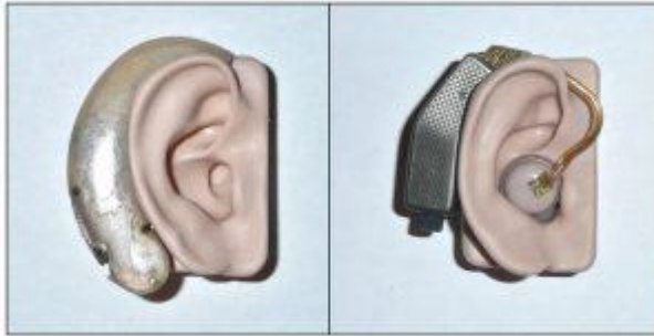
Figure 2. Zenith Diplomat introduced in 1956 (left aid), and the Dahlberg Magic Ear II introduced in 1957 (right aid). The size reduction in one year was rather remarkable. The Dahlberg aid would fit better on the ear had I chosen to reshape/change the receiver linkage. However, I try not to make any changes on any of the aids in my collection.
