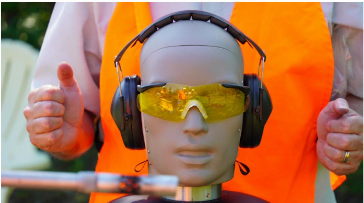
Figure 2. Earmuffs and ballistic safety glasses positioned on the acoustic test fixture (Position 1, 179 dB pSPL). The muzzle of the .300 caliber Browning A-Bolt rifle is shown in the foreground.
