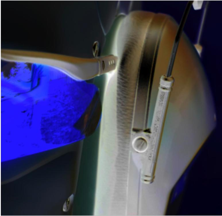
Figure 1. Close-up view of deformation of the earmuff cushion from the ballistic safety glasses resulting in an acoustic leak.
