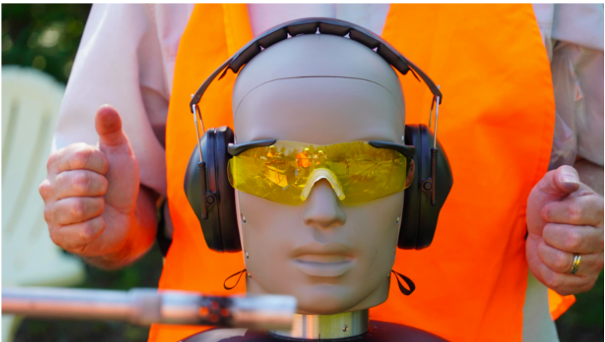
Figure 2. Earmuffs and ballistic safety glasses positioned on the acoustic test fixture (Position 1, 179 dB pSPL). The muzzle of the .300 caliber Browning A-Bolt rifle is shown in the foreground.
