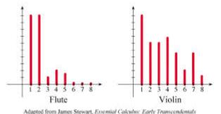
Figure 2. Despite both the flute and the violin being half wavelength resonator musical instruments and having their harmonics at exactly integer multiples of the fundamental, it is the relative heights of the harmonics that define their unique sounds.
