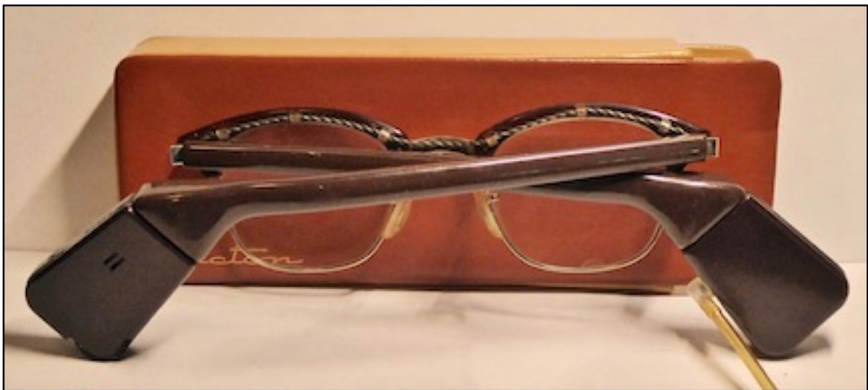
Figure 1. Dicton cross-head hearing aid from 1958. The microphone is on one side, along with the amplifier and power supply, and then wired through the eyeglass temple and frame to the opposite side to the hearing aid receiver where the sound is directed to the ear through plastic tubing to an earpiece. (From Staab Collection).
