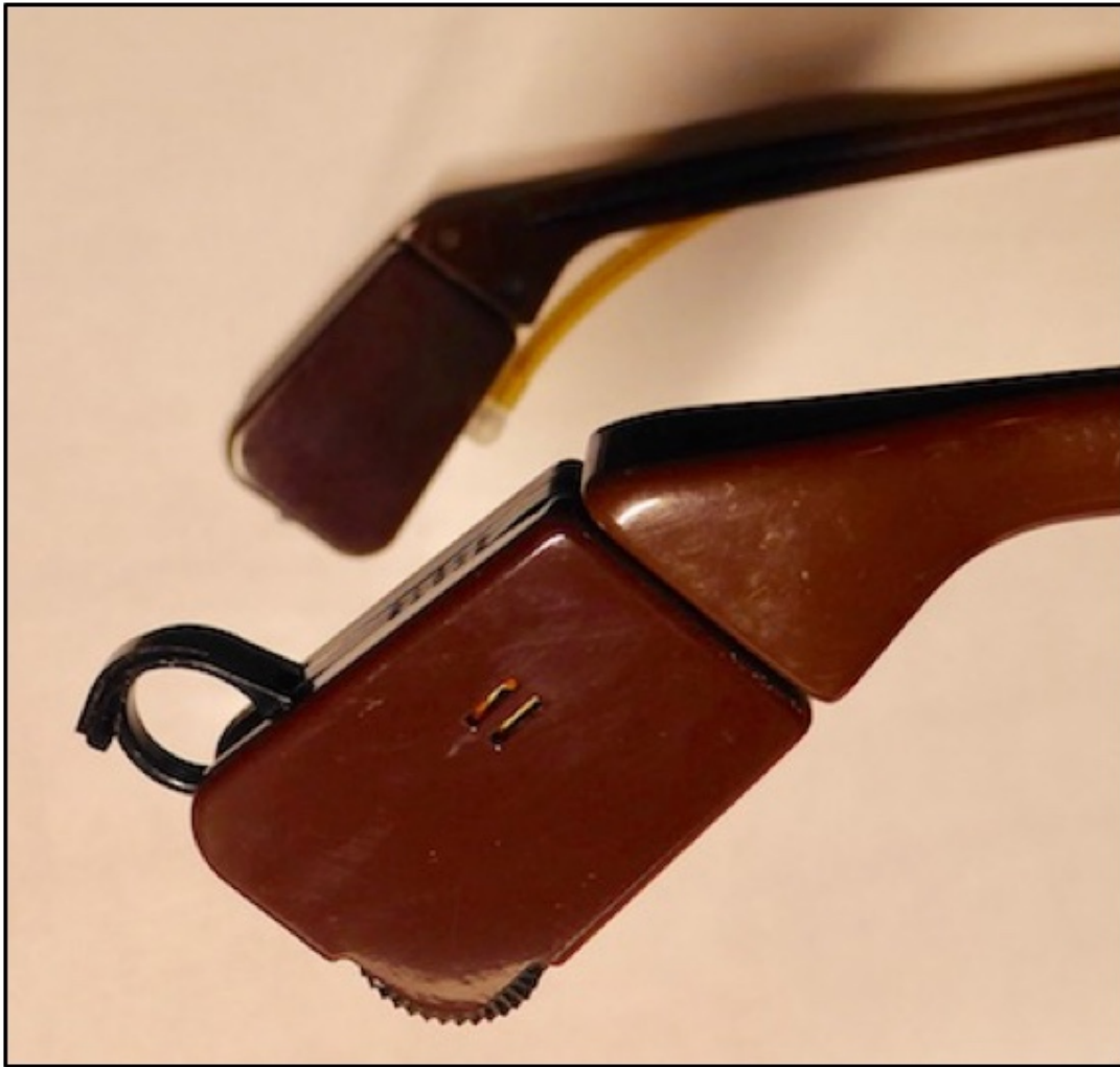
Figure 2. Microphone, power supply, volume control, and amplifier side shown closest. The two small slits are the microphone opening. The battery compartment is open to show its position. It used a 625 cell. The volume control is on the lower back and upon turning it, does not suggest that the volume control also has an ON/OFF switch. There were no other controls. The far image is the other side of the eyeglass hearing aid. That portion contained primarily the receiver. Sound was delivered to the ear through a polyethylene flexible tube ending in some kind of ear piece.
