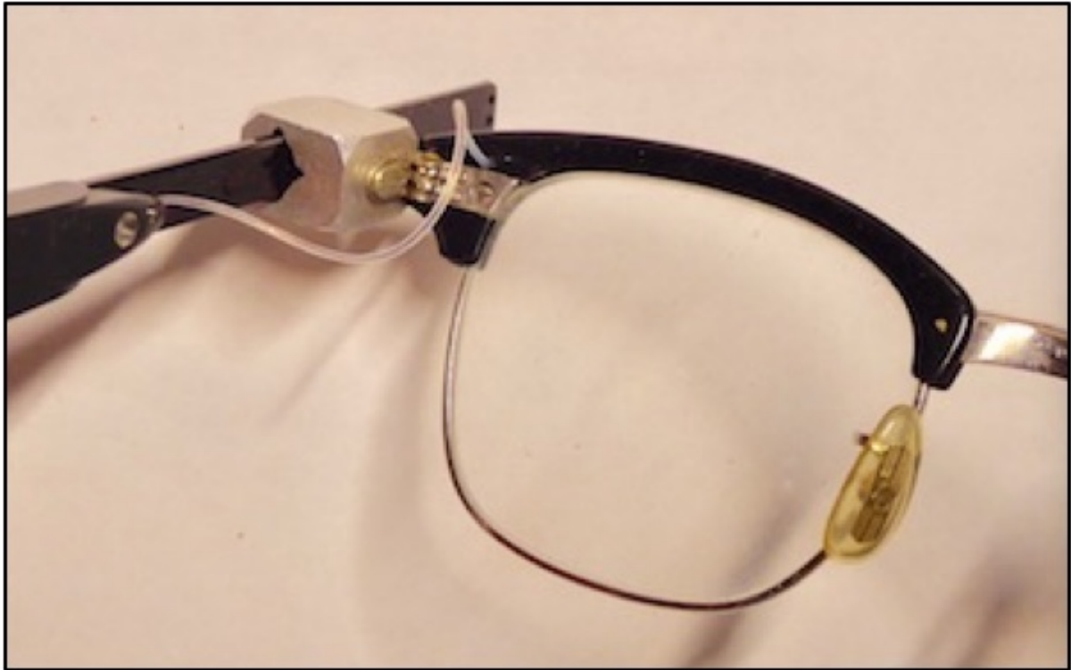
Figure 7. Later models of CROS eyeglass hearing aids used a wire arrangement very similar to that of the Diction unit. Some dispensers grooved the back of the top of the frame and placed the wires into that groove and covered it with some kind of sealer. At other times, an attempt was made to place the wires in the groove for the glass in the eyeglass frame. The metal piece that the temple slides through was used to determine the temple length.
