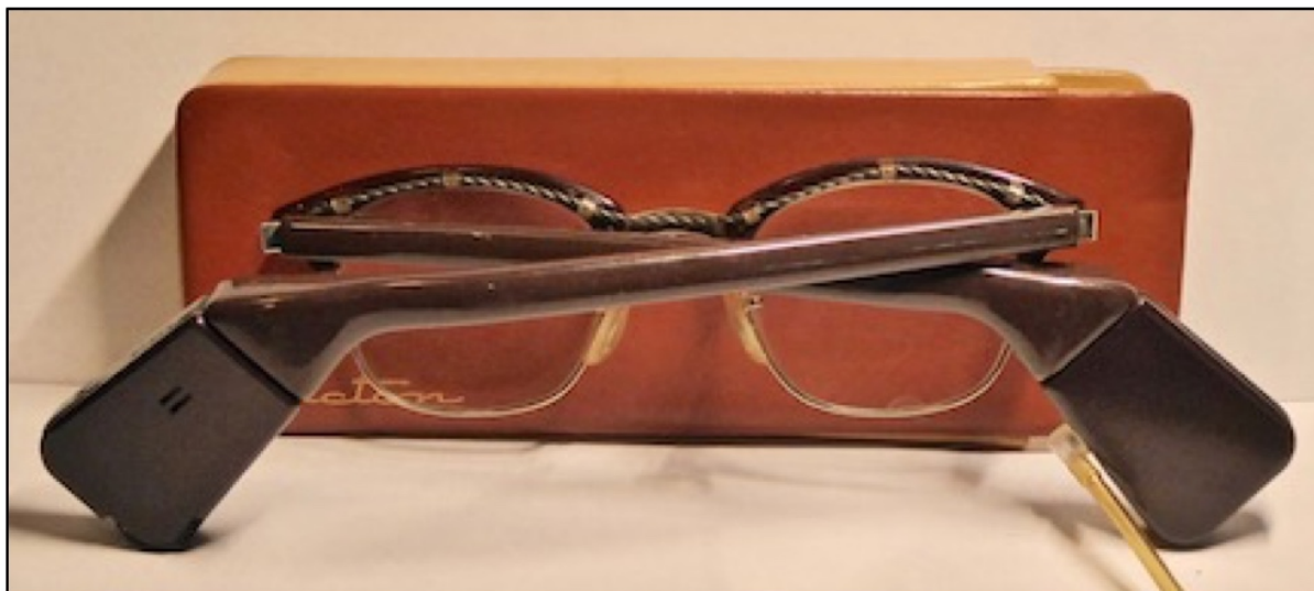
Figure 1. Diction cross-head hearing aid from 1958. The microphone is on one side, along with the amplifier and power supply, and then wired through the eyeglass temple and frame to the opposite side to the hearing aid receiver where the sound is directed to the ear through plastic tubing to an earpiece. (From Staab Collection).
