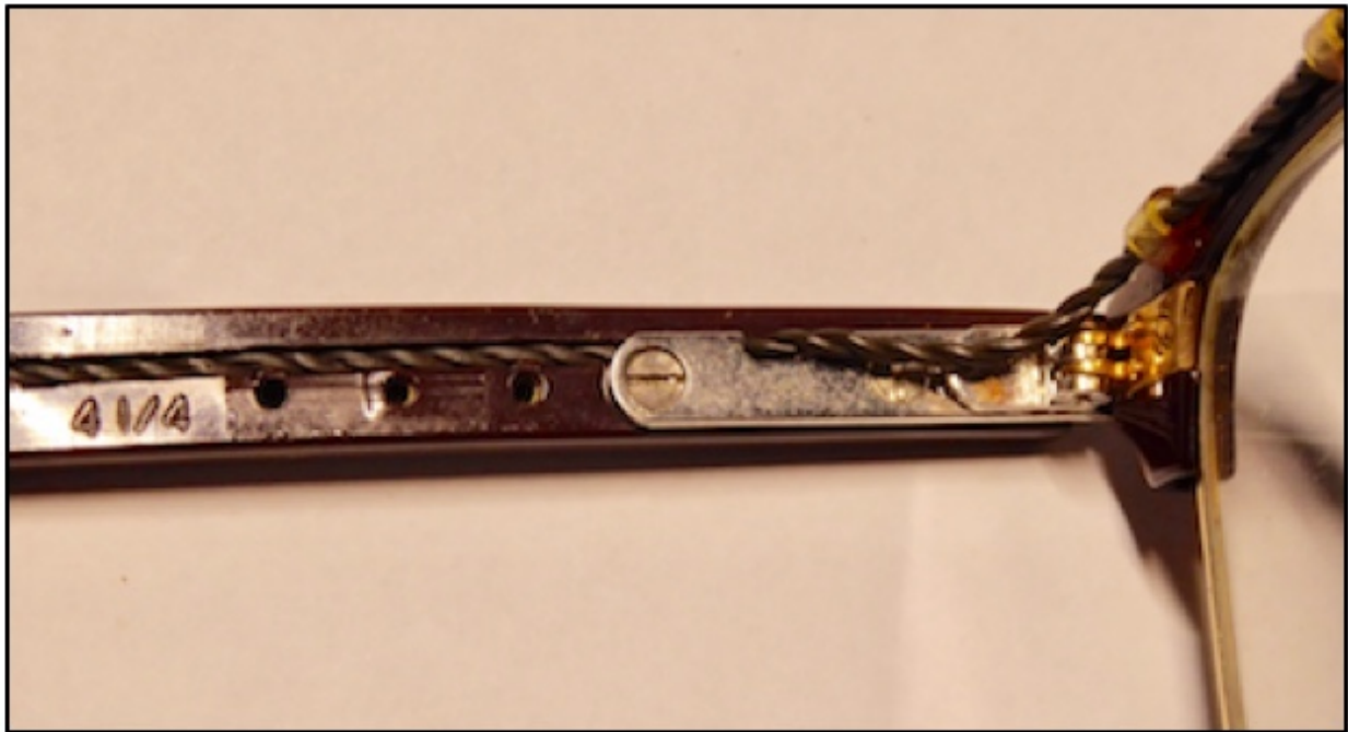
Figure 4. This image shows the wiring through the hinge connection and temple length adjustment. The temple was designed for 4 length adjustments down to 4 and \frac{1}{4} inches. The screws on the metal portion were moved to one of the 4 pre-drilled and threaded hole options and that part of the temple overlapping the front of the eyeglass was cut off.
