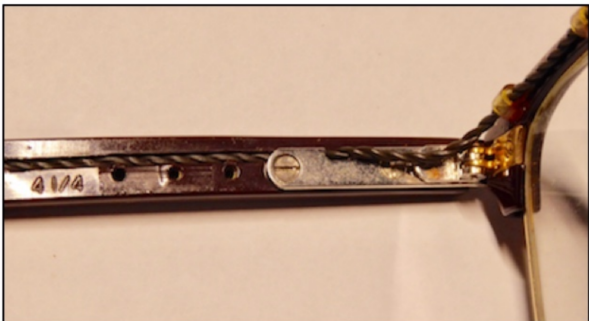
Figure 4. This image shows the wiring through the hinge connection and temple length adjustment. The temple was designed for 4 length adjustments down to 4 and ¼ inches. The screws on the metal portion were moved to one of the 4 pre-drilled and threaded hole options and that part of the temple overlapping the front of the eyeglass was cut off.
