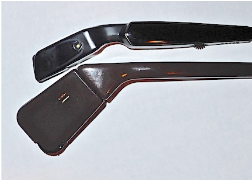
Figure 6. A Maico Transist Ear (top, about 1970 and Dicton (bottom, 1958). Aside from size resulting from components, the Dicton had its electronics all in the paddles, with some components in each paddle. The Maico had its amplification forward of that part of the temple that fit over the ear. The volume control wheel is seen at the bottom of the aid, and forward. The microphone remained in the paddle, as identified by the small whitish dot. Because this was a CROS hearing aid, the receiver is in the opposite ear temple. Wiring through the frame was often placed in the groove where the glass fits into the frame (Figure 7).
