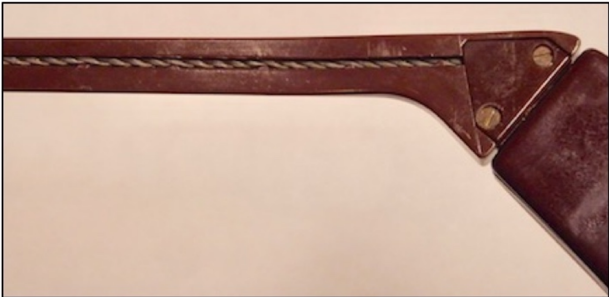
Figure 3. The wiring routing the signal from the microphone/amplifier side is fitted in a groove cut into both eyeglass temples. The plate (identified by the two screws) where the wire is hidden served also to store excess wire when the temple is shortened. No rewiring was required.
