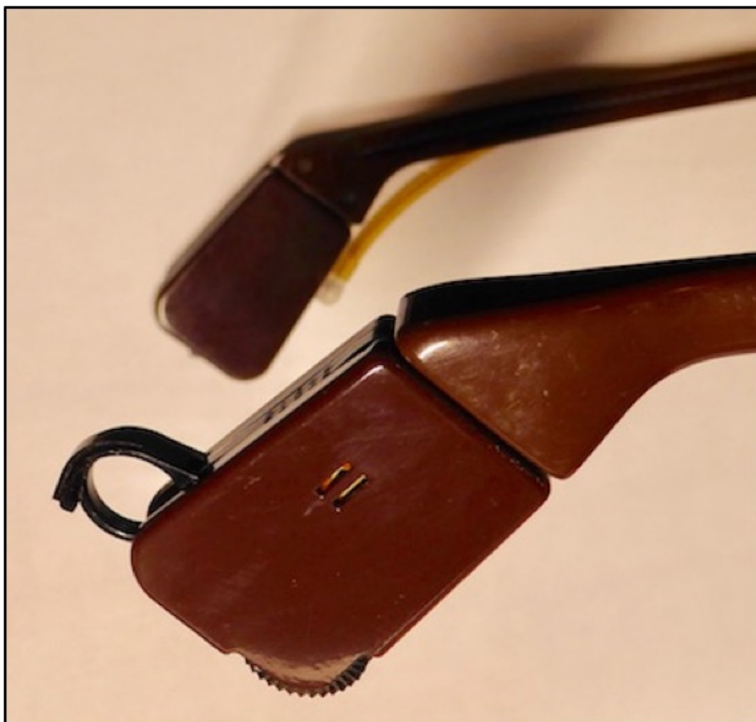
Figure 2. Microphone, power supply, volume control, and amplifier side shown closest. The two small slits are the microphone opening. The battery compartment is open to show its position. It used a 625 cell. The volume control is on the lower back and upon turning it, does not suggest that the volume control also has an ON/OFF switch. There were no other controls. The far image is the other side of the eyeglass hearing aid. That
