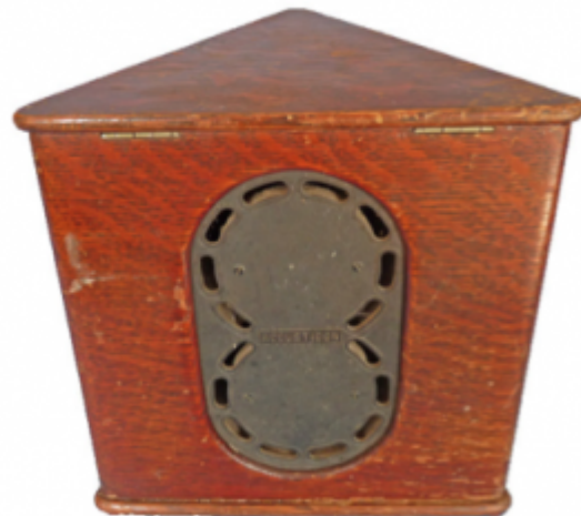
Fig 12. The Acousticon Dining Table Model carbon hearing aid had 6 microphones—2 on each side (1908- 1910).
