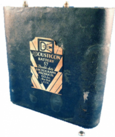
Fig. 29. The Acousticon No. 57 hearing aid battery—one of the largest hearing aid batteries made contrasted with the tiny Panasonic No. 5 battery—the smallest hearing aid battery made.
