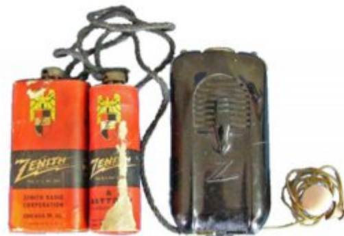
Fig. 18. The Zenith Model A3A-B3A “Radionic”—a two-piece vacuum-tube hearing aid. The large “B” battery is on the left and the round “A” battery beside it (1944).
