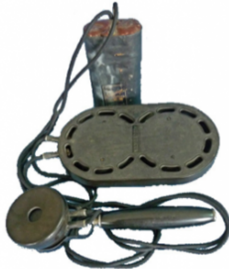
Fig. 14. The Acousticon Model SRD was a medium-powered double carbon microphone hearing aid. You could wear the double-carbon microphone around your neck or clipped to your shirt-front (1910 – 1928).
