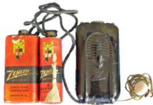
Fig. 18. The Zenith Model A3A-B3A “Radionic”—a two-piece vacuum-tube hearing aid. The large “B” battery is on the left and the round “A” battery beside it (1944).
