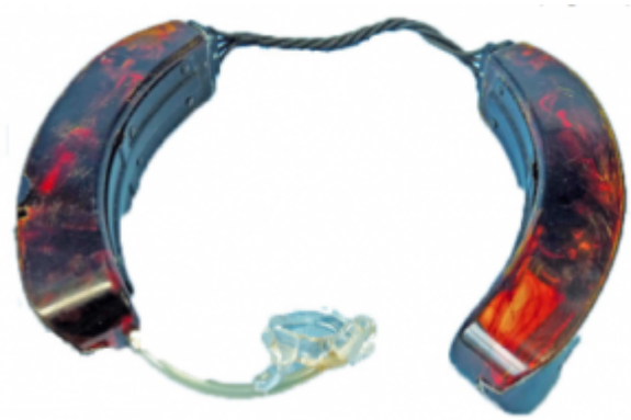
Fig. 20. Acousticon's Model A-200—a rare double-barrette vacuum-tube hearing aid for the ladies (1951).
