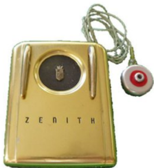
Fig. 23. The Zenith “Royal” vacuum-tube hearing aid was one of Zenith’s last vacuum tube hearing aids made (Feb, 1952).
