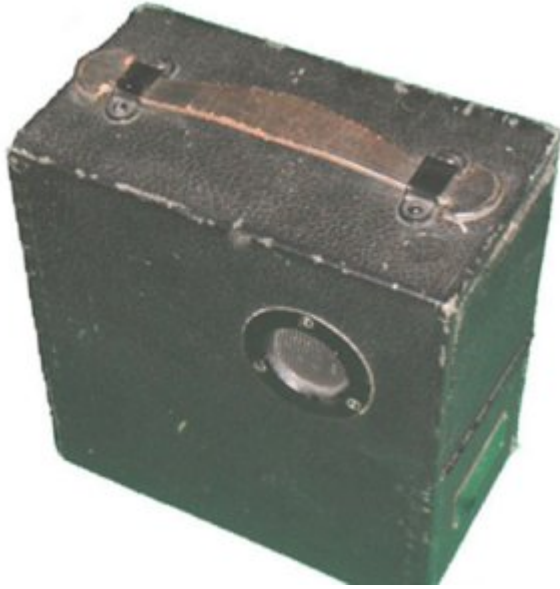
Fig. 17. The Globe “Vactuphone”—the first commercially- produced vacuum tube hearing aid (1921). This Vactuphone hearing aid still works after all these years. The tube is now 92 years old!
