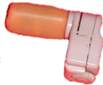
Fig. 26. The Telex Model 23 “Electron Ear”—an early ITE hearing aid (1965).
