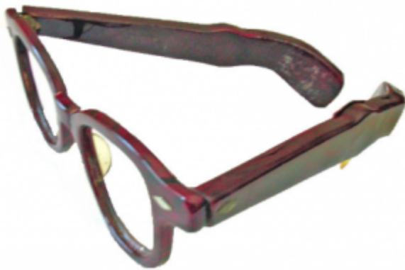
Fig. 27. The Otarion Model L10 “Listener”—the world’s first transistorized, eyeglass hearing aid (Dec, 1954).
