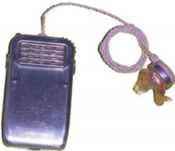
Fig. 21. Sonotone's Model 1010 hybrid (1 transistor & 2 vacuum tubes)—the first hearing aid in the world to use a transistor (Dec, 1952).
