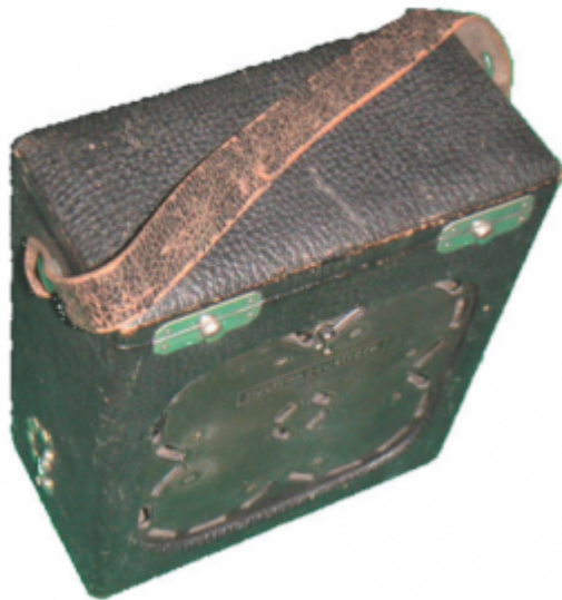
Fig. 15. The high-powered (4 microphone) Acousticon Model RF carbon hearing aid had a six-step volume control on the left end of the case to reduce the volume if it was too loud (1910 – 1923).
