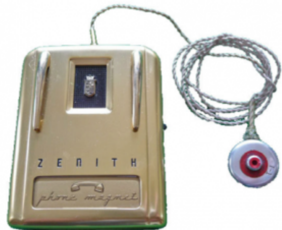
Fig. 24. The Zenith “Royal T” was Zenith’s first all-transistor hearing aid (Feb, 1953). It was the same size as the “Royal” vacuum-tube aid. Note that it had a t-coil built in—called a “phone magnet” in those days.
