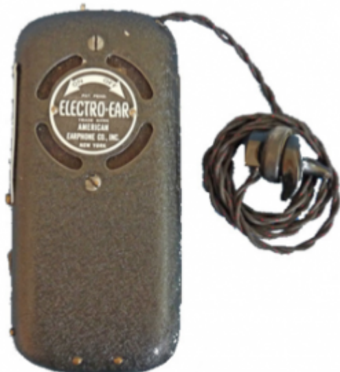
Fig. 16. The “tiny” Electro-Ear Model 5 wearable carbon hearing aid had internal batteries (c.1938).
