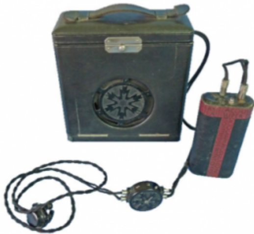
Fig. 13. The Acousticon Model 28 carbon hearing aid—a lower- powered single carbon microphone hearing aid shown in its resonant case (1927).
