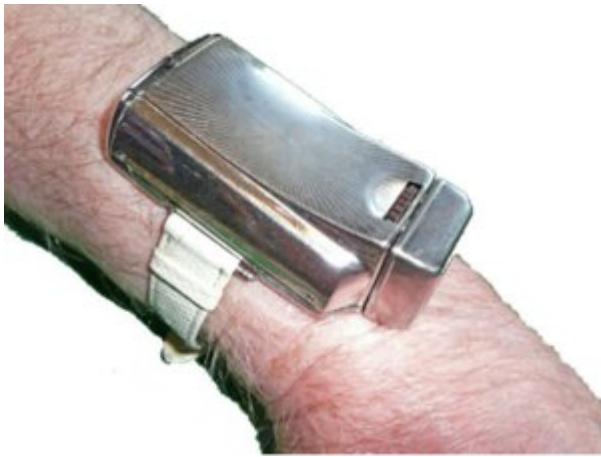
Fig. 19. Acousticon's Model A-165 was the only wrist-worn vacuum-tube hearing aid ever made (1950).
