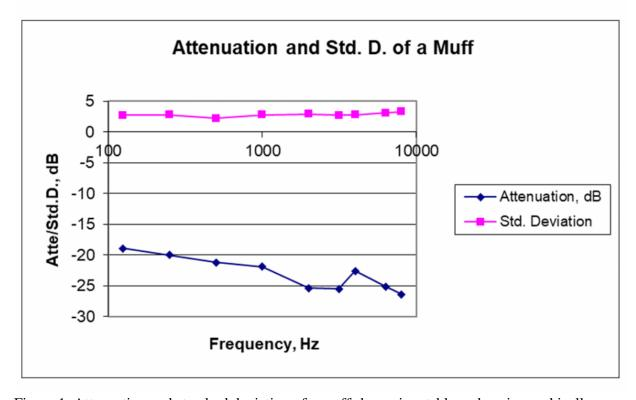
Figure 1. Attenuation and standard deviation of a muff shown in a table and again graphically.
