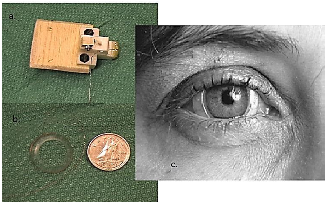
Figure 5. (a) the head coil (“bite block”); (b) scleral coil; (c) scleral coil on an eye.
