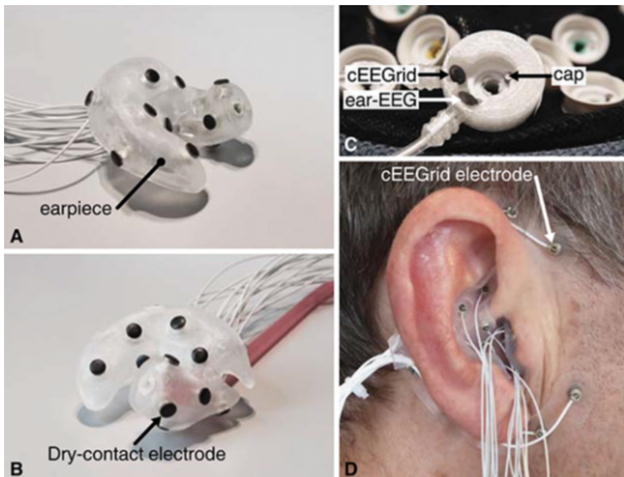
Figure 2. In- and around-ear EEG. Panel A and B show dry contact electrodes (black dots) throughout an ear piece. Panel C shows the sensor sizes in comparison to sensor mounts found on a typical EEG cap. D shows both a transparent around-ear montage (known as a cEEGrid) as well as the ear-EEG mould. Original image from Kappel, S. L., Makeig, S., & Kidmose, P. (2019). Ear-EEG forward models: improved head-models for ear-EEG. Frontiers in neuroscience , 13, 943. Reproduced here under CC BY International 4.0 license.
