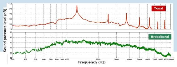
Figure 1. Spectra of the two reverse alarms.1
