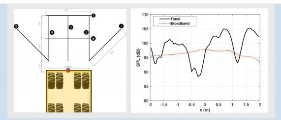
Figure 2. Sound propagation of reverse alarms behind a vehicle2. Left: measurement trajectories. Right: sound level distribution 2 meters on either side of the midline along trajectory 6 for the tonal (black line) and broadband (dotted line) alarms. The red dot represents the position of the alarm unit.
