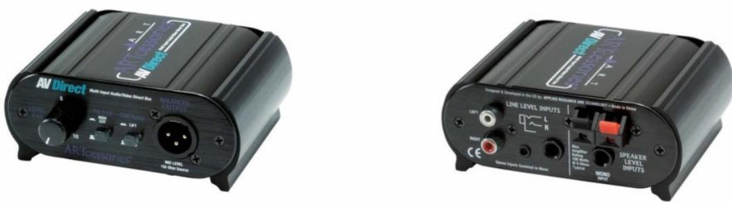
Figure 2 shows an AV-Direct box (ART manufacturer). At first glance, this looks like it has an RCA (unbalanced) INPUT to an XLR (balanced) OUTPUT which is the opposite of what we need. We required a method to convert a balanced OUTPUT from the console to the unbalanced INPUT of the Bluetooth accessory. And the connectors used - specifically the male XLR - reflect this standard of usage for this DI. We will turn this around... because a passive DI can work in both directions.
