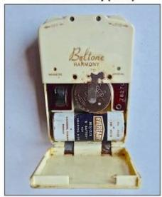
Figure 9. Beltone Harmony 3-vacuum tube hearing aid of 1946. This image shows the hearing aid with the round RM-4 "A" battery and a 30 volt "B" battery (in this case the Eveready 413E). This unit used a crystal microphone, as identified by the green dot on the right above the battery opening. The unit measured  $108 \times 70 \times 24$  mm.
