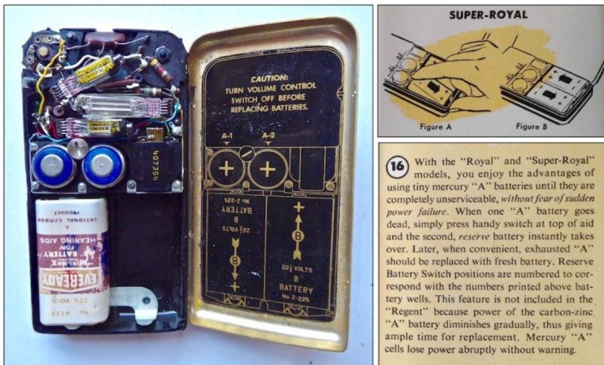
Figure 12. Zenith Super Royal 3 vacuum tube hearing aid of 1951. This hearing aid was unique in that it used four batteries. It had two “A” 1.5 volt batteries and two 22.5 volt “B” batteries, which were wired in series to produce 45 volts for added output power. It measured 113 x 59 x 22 mm in size. This shows the two RM-1 batteries in place, but only one of the 22.5 volt batteries.
