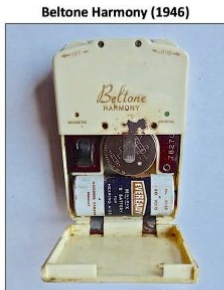
Figure 9. Beltone Harmony 3-vacuum tube hearing aid of 1946. This image shows the hearing aid with the round RM-4 “A” battery and a 30 volt “B” battery (in this case the Eveready 413E). This unit used a crystal microphone, as identified by the green dot on the right above the battery opening. The unit measured 108 x 70 x 24 mm.
