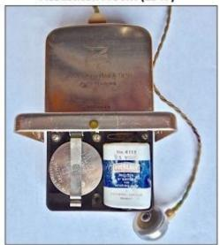
Figure 10. The Acousticon A 90M vacuum tube body-worn hearing aid of 1947 was made by Dictagraph Products of New York. This used a RM-4 "A" battery (1.5 V) and a 15 volt "B" battery. Although smaller that most previous body-worn hearing aids, it still measured 105 x 60 x 22 mm in size.
