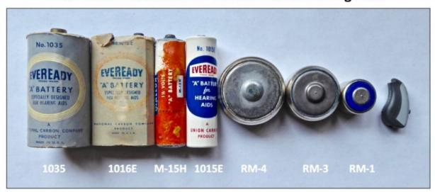
Figure 3. "A" battery size and shape examples used with vacuum tube hearing aids. Some were a button-type cell, as shown on the right. A 2017 behind-the-ear hearing aid is shown on the extreme right to provide a reference as to sizes. These are all 1.5 volt batteries used for vacuum tube hearing aids, not the 1.4 volt batteries used later in hearing aids using transistor circuitry.
