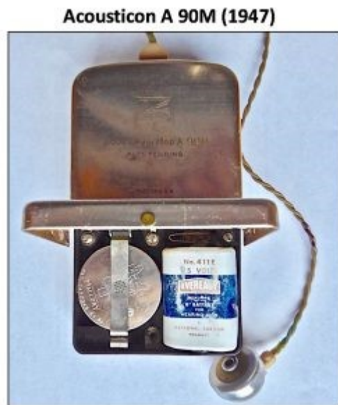
Figure 10. The Acousticon A 90M vacuum tube body-worn hearing aid of 1947 was made by Dictagraph Products of New York. This used a RM-4 “A” battery (1.5 V) and a 15 volt “B” battery. Although smaller than most previous body-worn hearing aids, it still measured 105 x 60 x 22 mm in size.
