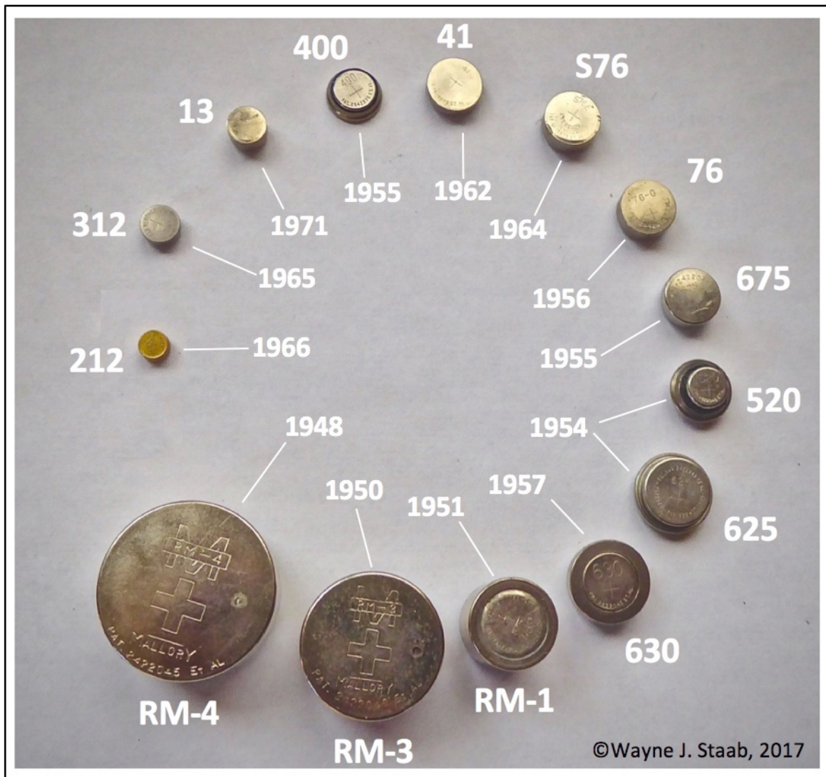
Figure 5. Shapes and size reductions in button cells used in hearing aids, with an attempt to show when they started being used in hearing aids. This is not a complete listing, but only features the most common. The three largest (RM-4, RM-3, and RM-1) are Mallory “A” button cells. To the right of these three “A” batteries, and curling around are the single power supply cells used following wide-spread user of transistors in hearing aids. These replaced both the “A” and “B” batteries. As single power supply cells, they no longer carried the designation of “B” batteries. None of these were zinc-air cells.
