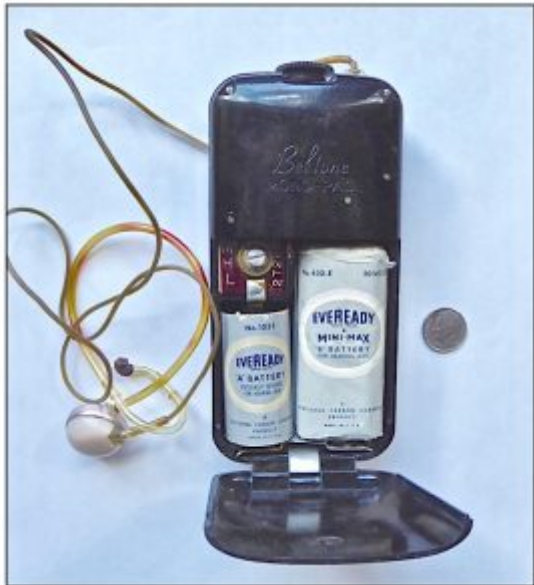
Figure 1. Beltone Monopac body-worn hearing aid (1944). This instrument captured all the hearing aid components into one case, with the exception of the receiver which delivered the signal via a cord to the ear. The monopac allowed for the user to carry one package, rather than two. Previous hearing aids had a separate pack for the batteries, and another for the hearing aid.
