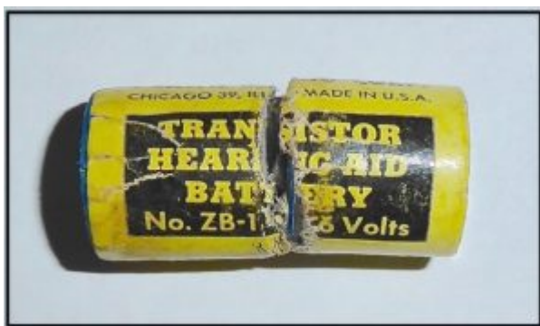
Figure 6. This Zenith ZB-1 (a guess based on the inability to determine what might have been printed in the space of the paper split) battery consists of two RG-1 (General Battery Co.) batteries
