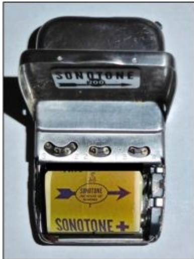
Figure 14. Sonotone 200 4-transistor body-worn hearing aid. This was powered by a 2.8-volt battery package. The controls above the battery were, from left to right: 4-position power control, 2-position low-pass filter, and a 2-position high-pass filter. These were adjusted by the hearing aid dealer.
