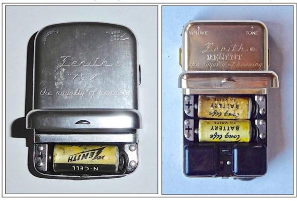
Figure 13. Early hearing aids that used the 401, 1.4-volt battery (Zenith N-Cell), were the Zenith "75-X" and the Zenith "Regent." The reason for the two batteries related to the output power, with the "Regent" providing a very high output of 142 dB SPL.
