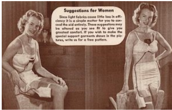
Figure 8. Battery pack suggestions for women as provided by Zenith Radio Corporation for its A2A body-worn hearing aid owner's manual.
