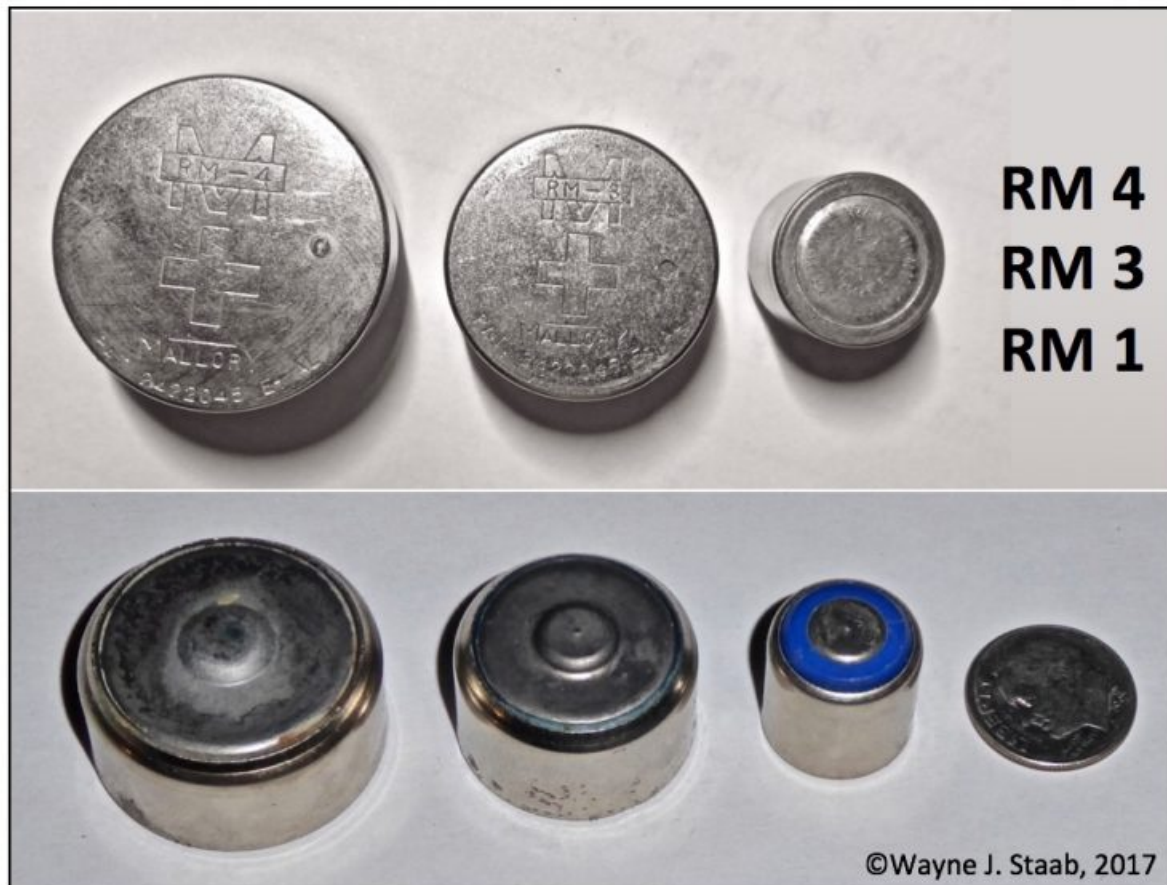
Figure 4. Mallory RM button batteries. These were all 1.5 volts and were used as the “A” battery in many hearing aids in the late 1940s and early 1950s. The RM-4 was the largest button battery made for hearing aid use. It weighed 1.6 oz. (45 grams) and measured 30 mm in diameter and had a height of 17 mm. The RM-3 was 25 mm in diameter and had a height of 16 mm. It weighed 1 oz. (30 grams). The RM-1 measured 15.5 mm in diameter and had a height of 16 mm. It weighed 0.4 oz. (10 grams). It is not clear if a RM-2 existed for hearing aids. A very small hole on the positive side of the RM-4 and RM-3 acted as a valve to relieve excess pressure that could be built up when the battery was being used. The bottom images represent the underside of the batteries shown on the top section.
