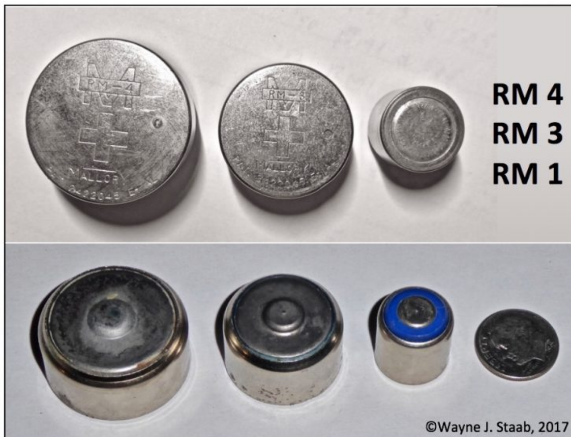
Figure 4. Mallory RM button batteries. These were all 1.5 volts and were used as the “A” battery in many hearing aids in the late 1940s and early 1950s. The RM-4 was the largest button battery made for hearing aid use. It weighed 1.6 oz. (45 grams) and measured 30 mm in diameter and had a height of 17 mm. The RM-3 was 25 mm in diameter and had a height of 16 mm. It weighed 1 oz. (30 grams). The RM-1 measured 15.5 mm in diameter and had a height of 16 mm. It weighed 0.4 oz. (10 grams). It is not clear if a RM-2 existed for hearing aids. A very small hole on the positive side of the RM-4 and RM-3 acted as a valve to relieve excess pressure that could be built up when the battery was being used. The bottom images represent the underside of the batteries shown on the top section.
