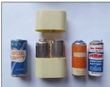
Figure 15. Examples of smaller batteries used with transistor hearing aids. On the left is a General mercury 2.6-volt battery. The plastic-shelled battery in the center is actually two 401 (1.4 volt) batteries soldered together to generate a series connection to provide 2.8 volts. An example of this was the Sonotone 600 battery. It generated 2.8 volts. The two batteries on the right were early 401 (1.4 volt) mercury batteries for transistor hearing aids by Mallory and Eveready.
