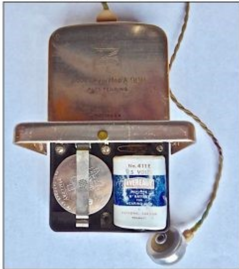
Figure 10. The Acousticon A 90M vacuum tube body-worn hearing aid of 1947 was made by Dictagraph Products of New York. This used a RM-4 “A” battery (1.5 V) and a 15 volt “B” battery. Although smaller than most previous body-worn hearing aids, it still measured 105 x 60 x 22 mm in size.
