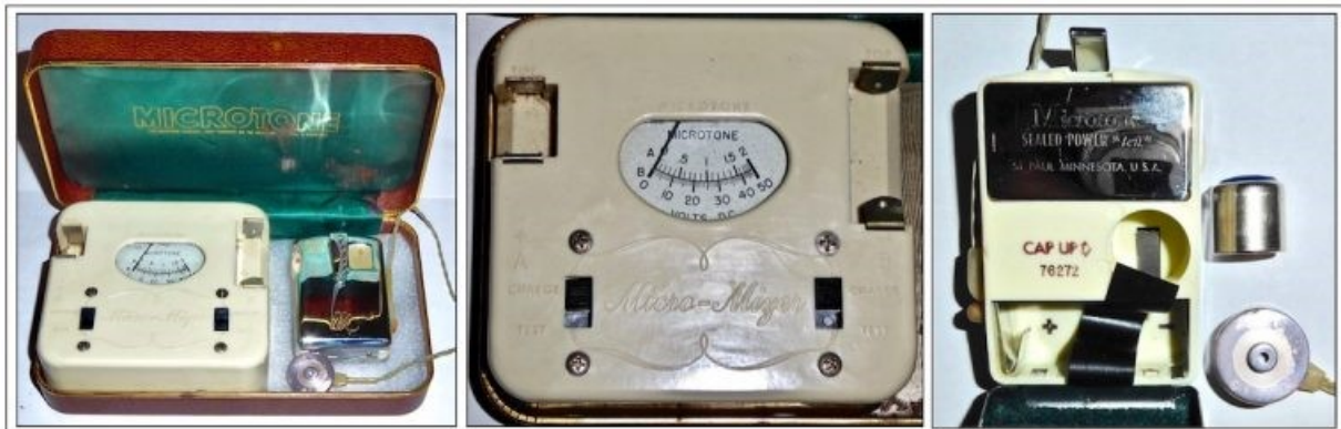
Figure 11. Microtone T-10 Sterling Silver hearing aid and its “Micro-Mizer” A/C powered battery tester. The battery tester had two slots for testing and reconditioning the two different hearing aid batteries. Their voltages were measured on the same voltage scale on the meter. It had a scale for the “A” battery and another for the “B” battery. Each was tested separately using a “Test” button on the tester. The range of the “A” battery was from 0 to 2 volts. That for the “B” battery ranged from 0 to 50 volts. The Micro-Mizer was used to place the batteries in overnight to “recondition” following daily use. It was advertised that by doing so, the effective life of the “A” battery could be extended by 3 to 4 times, and the “B” battery up to 5 times its normal life. It was recommended that the user have two sets of batteries so that one set could be “reconditioned” while the other set was being used.
