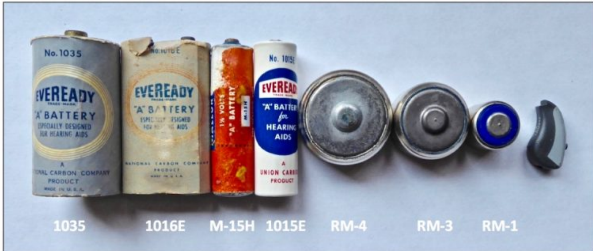
Figure 3. “A” battery size and shape examples used with vacuum tube hearing aids. Some were a button-type cell, as shown on the right. A 2017 behind-the-ear hearing aid is shown on the extreme right to provide a reference as to sizes. These are all 1.5 volt batteries used for vacuum tube hearing aids, not the 1.4 volt batteries used later in hearing aids using transistor circuitry.
