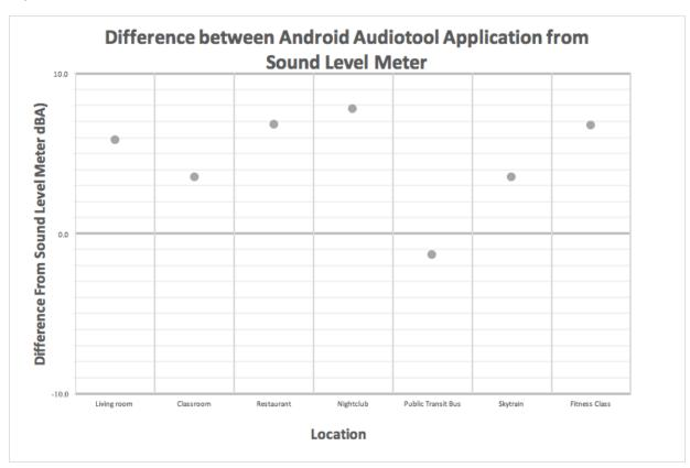
Figure 3. Android Audio Tool vs. SLM measurements.
