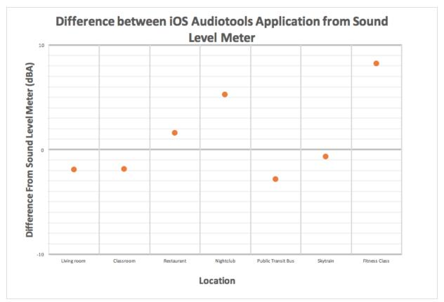
Figure 2. iOS AudioTools vs. SLM measurements.
