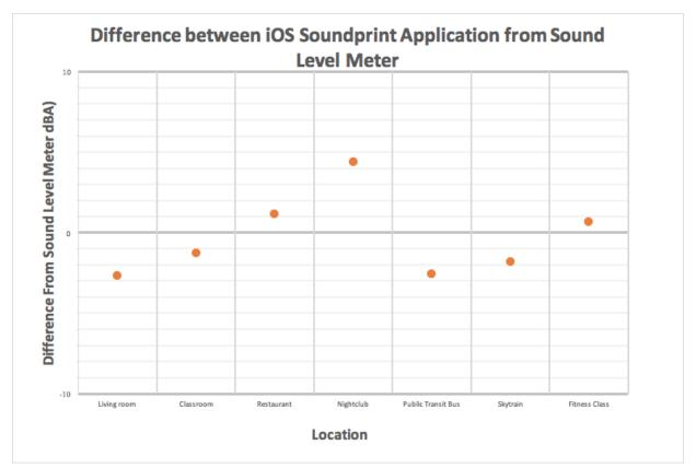
Figure 4. iOS SoundPrint vs. SLM measurements.
