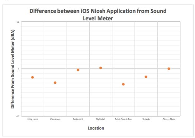
Figure 5. iOS NIOSH vs. SLM measurements.
