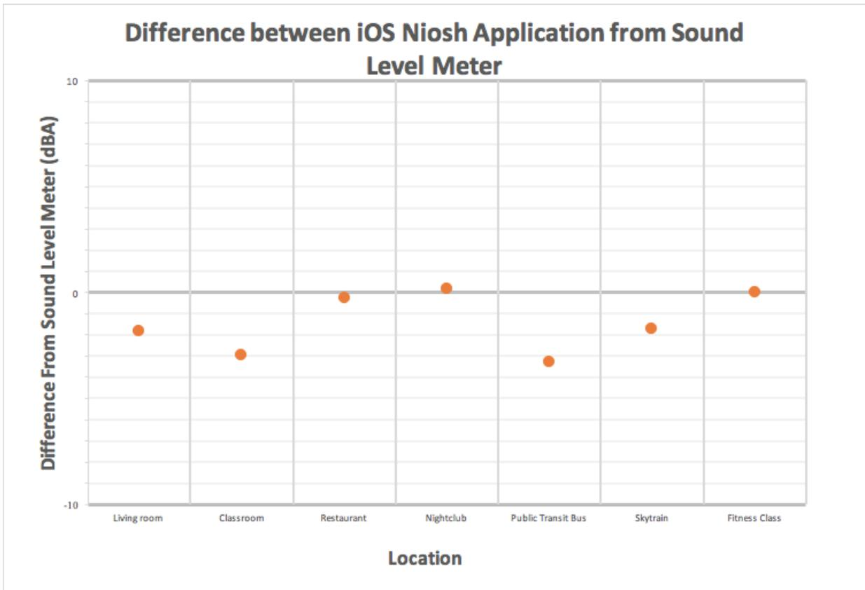
Figure 5. iOS NIOSH vs. SLM measurements.
